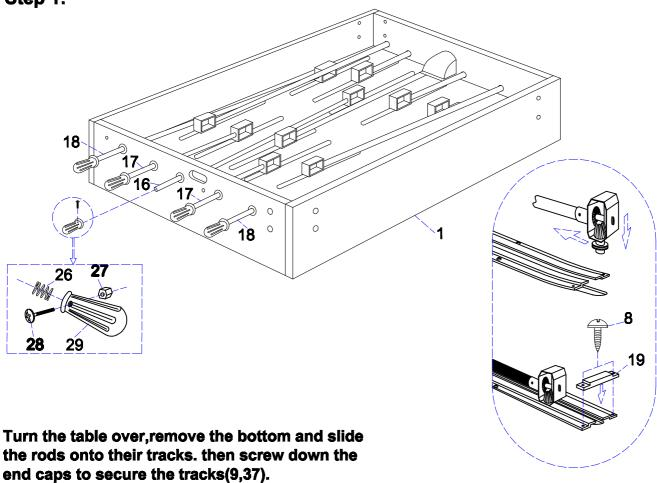
Then add the handles by sliding on a spring to the rod, sliding on the handle and bolting them to the rod(5,29,26,4).
